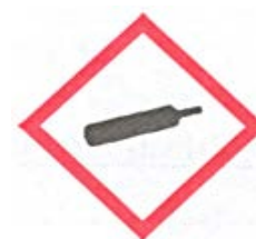
Gas under pressure
